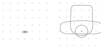
AG04 Symmetric Elliptical 17° - 46°
